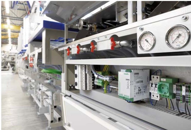
FIGURE 1: Kolbus GmbH & Co. KG from Rahden (Germany), a market leader in the area of bookbinding machines, deploys multiple distributed power supplies located at the main load points
