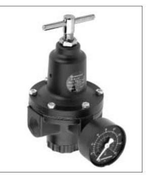
Ordering Information. Models listed have PTF threads, T-bar adjustment, relieving diaphragm, and 5 to 125 psig (0.3 to 8.5 bar) outlet pressure adjustment range\*.
