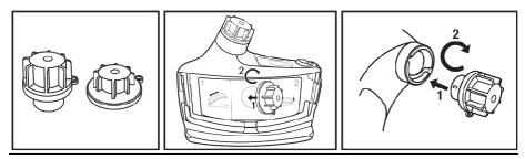
Figure 1. Installing the inlet and outlet plugs from the TR-653 Cleaning and Storage Kit
