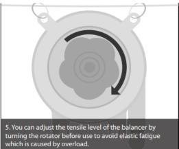
Counter clockwise rotation for a tension increase;
