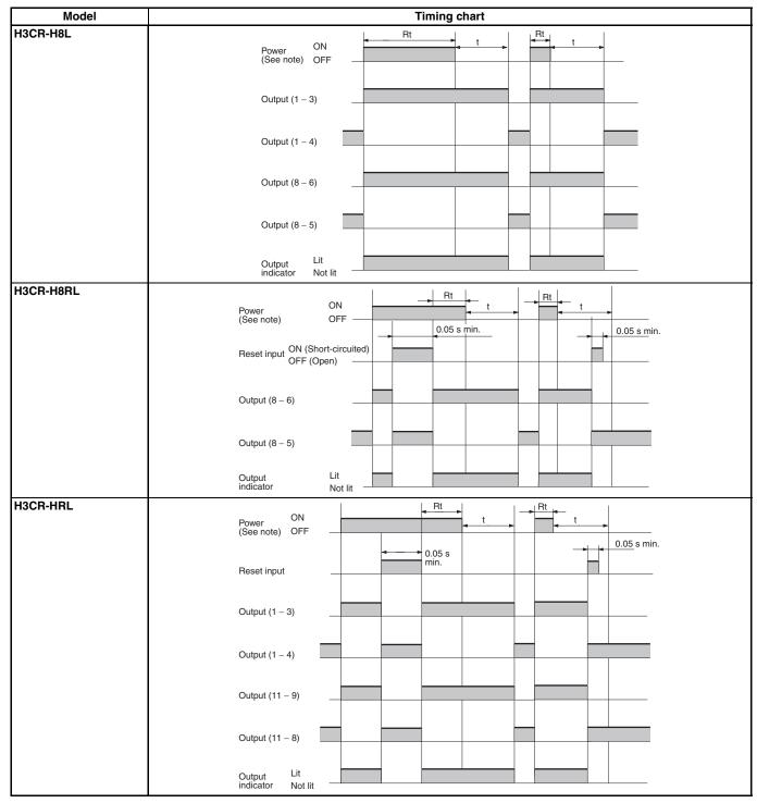
Note: If the power is turned ON until the set time is up, the timer will be retriggered.
