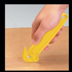
Turn handle over to cut tape between box flaps safely and effortlessly. Just poke through then pull in the direction of cut.
