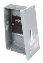
Siemens Energy Management Residential Specialty Load Centers: Small Circuit (2-10). Sub Brand: Load Centers Type: 1: Application: Residential: Voltage Rating: 120/240V Amperage Rating: 60A Phase: 1PH Load Regulation: 60A Wiring Configuration: 3w Bus Rating: 60A Interrupt Rating: 100000AIC. EQ LC 2S 4C ML 60A N1-S
