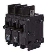
Siemens Low Voltage Molded Case Circuit Breakers General Purpose MCCBs are Circuit Protection Molded Case Circuit Breakers. 3-Pole Common-Trip circuit breaker type BQ. Rated 240 V (030A) (AIR 10 kA). Special features: line side lugs included. Note: Load side lugs are included.
