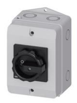
SENTRON, Switch disconnector 3LD, main switch, 3-pole, lu: 25 A, Operating power / at AC-23 A at 400 V: 9.5 kW, molded-plastic encapsulation for inch cable gland, rotary operating mechanism, black
