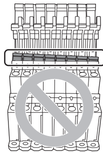
Incorrect installation Some terminals not inserted completely.
