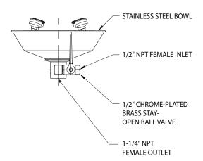
NOTE: EACH GS-PLUS SPRAY HEAD HAS A "FLIP-TOP" DUST COVER, INTERNAL FLOW CONTROL AND FILTER TO REMOVE IMPURITIES FROM THE WATER FLOW.
