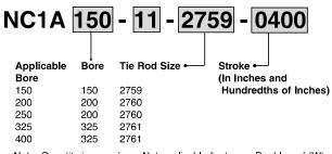
Note: Quantity is one piece. Not applicable for types: Double rod (W), Trunnion (T), XC8, XC9, XC10, XC11, Over sized rod (XB5) with front mounts. Please consult your local SMC sales office.
