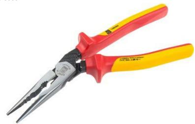
RS Pro VDE Long Nose Pliers, offers quality steel hardened and tempered with cutting edges separately induction hardened. Ergonomic angled head and handles for performance. Designed to keep a tight grip and pipe holes can grip different diameters while wave profile in the jaws gives ideal grip of softer materials.
