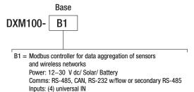
Outputs: (4) NMOS OUT, (2) analog OUT (0-10 V or 4-20 mA) Power Out: (2) Selected 5 V or 16 V switched power,
