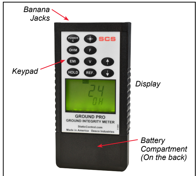
Figure 2. Ground Pro Meter features and components
