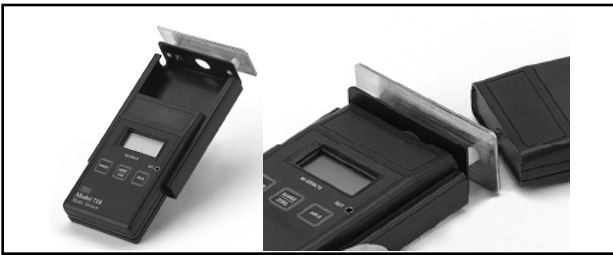
Figure 6. 718 Static Sensor charging plate in use.
