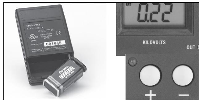
Figure 2. SCS 718 and 718A Battery Replacement and Indicators.
