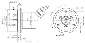
Order example for 6 mm shaft diameter: AHx36I-S3xx0xxxxx + BEF-FA-020-050-I (adapter is not pre-assembled) Solid shaft, face mount flange with flange adapter, centering collar D20 on D24 (BEF-FA-020-024-I, 2103982)
