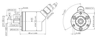
Order example for 6 mm shaft diameter: AHx36I-S3xx0xxxxx + BEF-FA-020-036-2-I (adapter is not pre-assembled)
