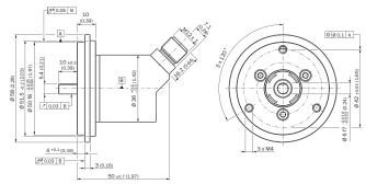
Order example for 6 mm shaft diameter: AHx36I-S3xx0xxxxx + BEF-FA-020-050-I (adapter is not pre-assembled) Solid shaft, face mount flange with flange adapter, centering collar D20 on D24 (BEF-FA-020-024-I, 2103982)
