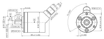
Order example for 6 mm shaft diameter: AHx36I-S3xx0xxxx + BEF-FA-020-036-2-I (adapter is not pre-assembled)
