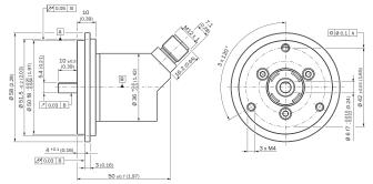
Order example for 6 mm shaft diameter: AHx36I-S3xx0xxxx + BEF-FA-020-050-I (adapter is not pre-assembled) Solid shaft, face mount flange with flange adapter, centering collar D20 on D24 (BEF-FA-020-024-I, 2103982)
