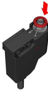
Figure 15. Install a new plastic washer
