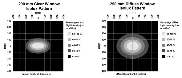
Lux and irradiance values shown are typical at 25 °C and with clear windows; light intensity lowered by 40% on diffuse window models.
