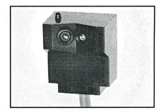
Leakage current and saturation voltage are both very low for easy interfacing to PLCs and other solidstate circuitry, including Banner logic modules (see hookup information). ECONO-BEAMs are protected against false pulse on power-up and voltage polarity reversal. A red indicator LED on top of the sensor lights whenever the ECONO-BEAM senses its own modulated light.
