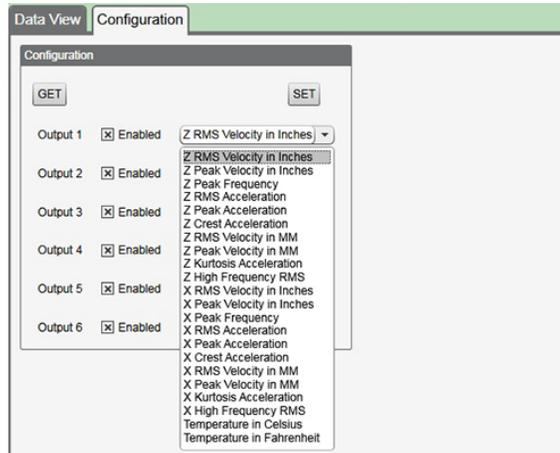
When the **Configuration** screen opens, click **GET** to read the current configuration from the Vibration/Temperature sensor into the software. The outputs listed on the screen are the sensor's outputs. Up to six sensor outputs may be mapped to the Node's inputs. The sensor's output 1 is automatically mapped to the Node's input 1.
