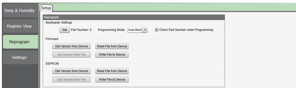
**Write File to Device.** To write firmware or EEPROM files to the sensor, follow these steps:
