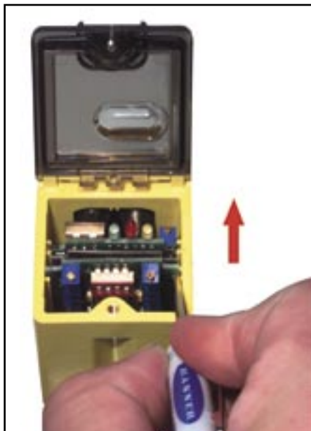
Figure 6. Using the small screwdriver in the module slot if necessary to nudge the module loose, lift the module up and out.
