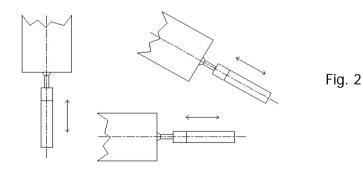
Rotate the SENSING HEAD is prohibited. Some certain angles between SENSING HEAD & measuring object are not allowed
