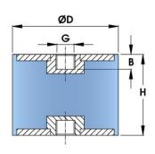
A simple and cost-effective mount. For use in compression and shear. A very large range of available size and studs.
