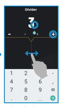
To change the value: Touch "3" and digit via keypad the correct value, or... Swipe horizontally, or... Touch + or - to change by 1, or touch **♣** or **■** to change by 10
