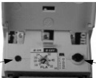
Overload Relay with Cover Open — FLA/Trip Class/Phase Protection Dial
