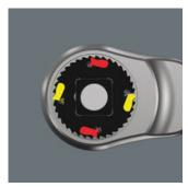
dual-ratchet-teeth design The means that a 76 fine-toothing division can be achieved from the 38 robust teeth with a return angle of only 4.7°.
