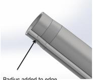
Radius added to edge to prevent wires from being cut
