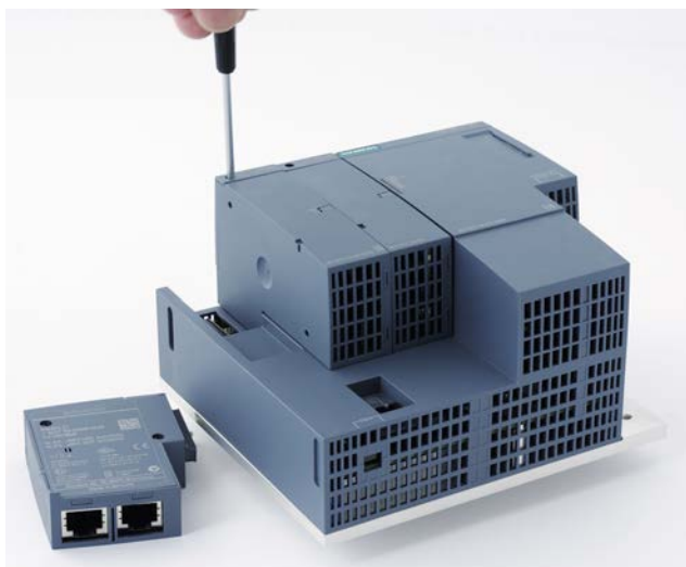
Figure 4-10 Installation of the modules
