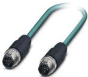
Assembled Ethernet cable, CAT5e, shielded, 2-pair, AWG 26 stranded (7-wire), RAL 5021 (sea blue), M12 plug to M12 plug, line, length 5 m
