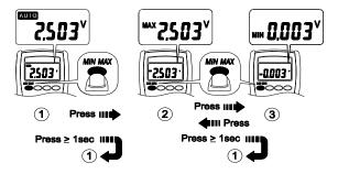
Note - Press the *HOLD* button in *MIN MAX* mode to make the meter stop updating the maximum and minimum value. When display *Hold* mode is nested in *MIN MAX* mode, the *MIN MAX* mode must be released before the display Hold.
