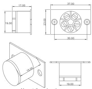
Magnet dimensions the same as switch dimensions except depth 15mm
