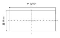
\*Panel thickness should be maximum 7mm.
