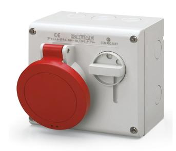
RS Pro surface mount interlock sockets feature a hard plastic housing and a socket cover. This range features a mechanical interlock that prevents the switch from closing when the plug is not inserted and prevents the extraction of the plug if the switch is closed. They are designed for industrial use, but are also suitable for commercial environments.
