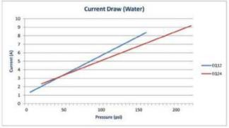
Pressure shown is the not to exceed value. All MG2000 pump variants are capable of more than the indicated figure but exceeding this may result in damage to the pump.
