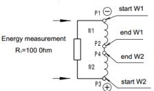
Observing the polarity a positive pulse is induced at press actuation and a negative pulse is induced at release actuation
