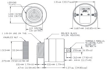
NOTE A: TERMINALS-.032 BRASS TIN PLATED, TAPPED FOR #6-32 SCREW. TWD #6-32 NICKEL PLATED BRASS SCREWS INCLUBED, WILL ACCEPT 1/4\* QUICK CONNECT. NOTE B: MOUNTING- REMOVE BLACK PLASTIC NUT AND INSERT THREADED FRONT THROUGH 1.25' HOLE PUNCHED IN PANEL, IF DRIENTATION IS NEEDED, NOTE LOCKING FLATS ON DRAWING. SCREW NUT BACK ON. DO NOT OVERTIGHTEN.
