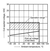
4. Ambient temperature characteristics (Cold/initial)
