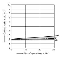
8-(2). Electrical life test (Halogen lamp load) Sample: CM1aF-R-12V, 6pcs.
