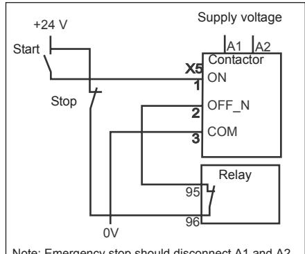
When used with switches the wiring can be done according to diagram above.
