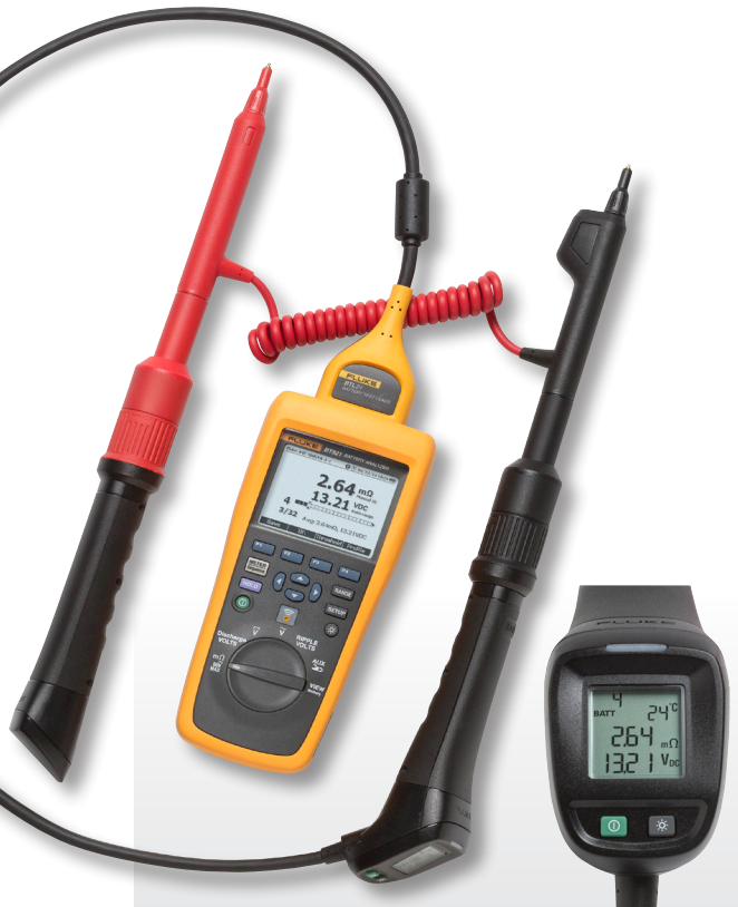
Intelligent test probe with integrated LCD display
