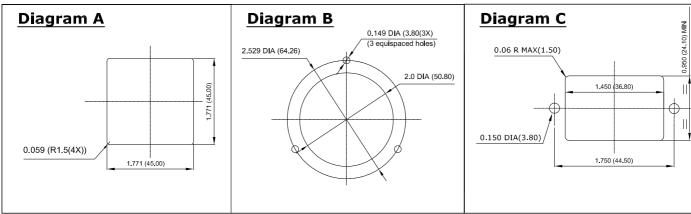
Max. Panel Thickness; 1.129 (0.76) to 0.401 (10.20) Panel Cut-out dimensions - Tolerance +/- 0.010 (0.30) All Dimensions are in inches, Values in () = mm
