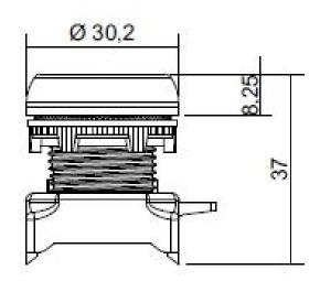
Illuminated flush pushbutton heads for use with the RS pro modular plastic push button series. Robust design in a variety of colours with modern aesthetics delivered via silver coloured bezel. Simple installation via standard lock nut.
