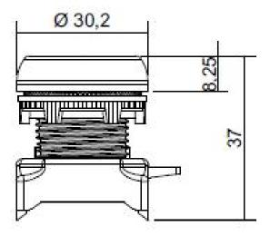
Printed flush push button heads for use with the RS pro modular plastic push button series. Robust design in a variety of colours and markings with modern silver coloured bezel. Simple installation via standard lock nut.
