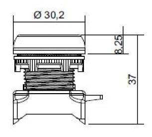
Non-illuminated flush push button heads for use with the RS pro modular plastic push button series. Robust design in a variety of colours with modern silver coloured bezel. Simple installation via standard lock nut.
