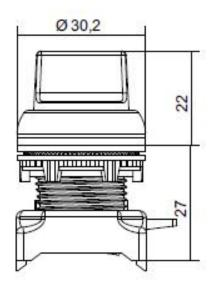
Selector switch heads in 2 and 3 position versions for use with the RS pro modular plastic push button series. Robust design with modern aesthetics delivered via silver coloured bezel. Simple installation via standard lock nut.
