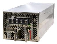
The TPS series industrial AC-DC power supplies offer output power up to 4,080W in a 2U high package with 3 phase supply input. Features include voltage and current programming, remote on/off, remote sense, a standby supply, PMBus communication, built in ORing FET and wide operating temperature range of -40°C to +70°C. The TPS4000 is also designed to meet MIL-STD-461F/G RE102 EMI and MIL-STD-810F vibration and shock.
