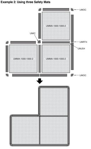
In this case, the perimeter of the Safety Mat is about 8 m, the joint between the Safety Mats is 2-m long, and the following pieces are required:
