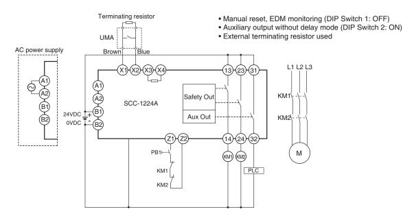
S1: Reset switch KM1, KM2: Magnetic contactor M: Motor
