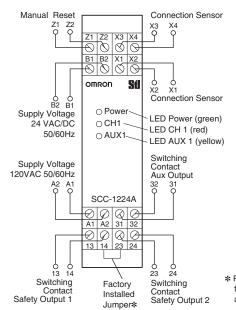
\* Remove the factory-installed jumper between terminals 14 and 23 if safety outputs 1 and 2 are not connected in series.
