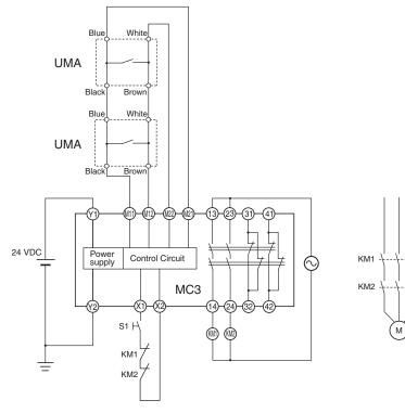
S1: Reset switch KM1, KM2: Magnetic contactor M: Motor
