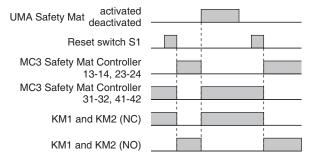
Note: Remove the three yellow jumpers from the MC3 to use Manual Reset Mode. Refer to *Changing the Reset Mode* on page 10 for the location of the jumpers.
