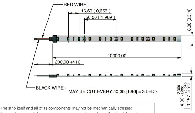
Assembly must not damage or destroy conducting paths on the circuit board. Correct electrical polarity needs to be observed, wrong polarity may destroy the strip. When mounting on a metallic or otherwise conductive surfaces, there needs to be electrical isolation points between strip and the mounting surface.
